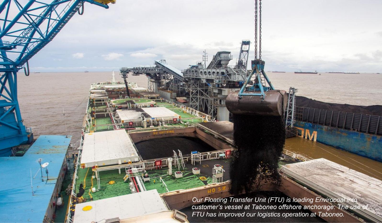
*Our Floating Transfer Unit (FTU) is loading Envirocoal into customer's vessel at Taboneo offshore anchorage. The use of FTU has improved our logistics operation at Taboneo.*
