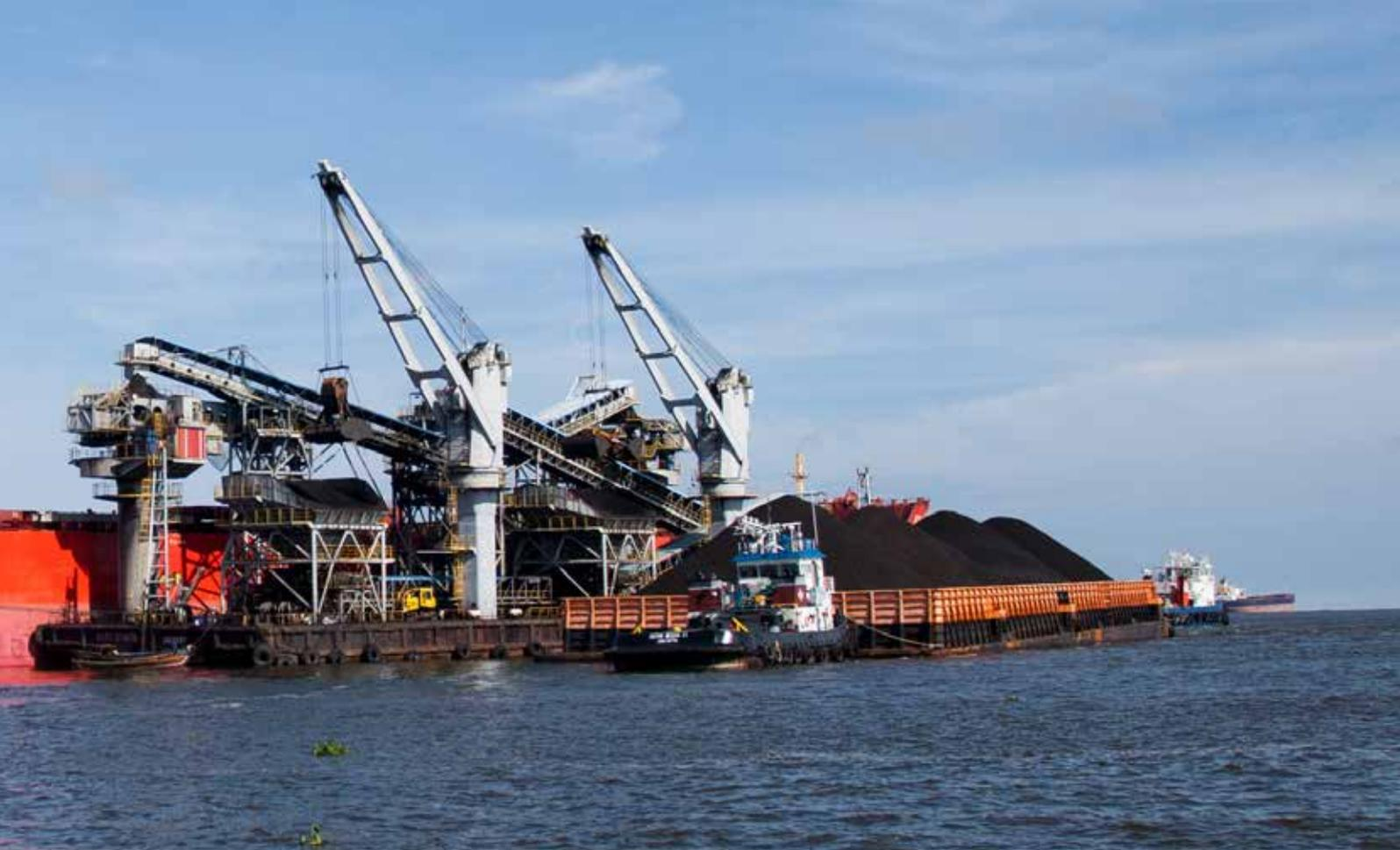
Situation in Taboneo Open Sea Anchorage, the coal is transferred from a barge to a buyer's vessel.
