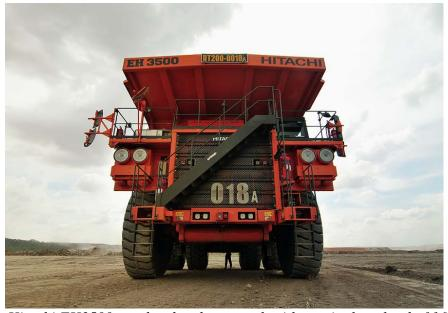
Our new Hitachi EH3500 overburden dump truck with nominal payload of 168 tonnes
