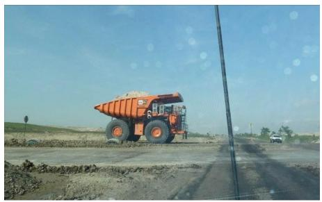
Our new and first electric dump truck with capacity of 170 tonnes to improve productivity and reduce operating and maintenance costs
