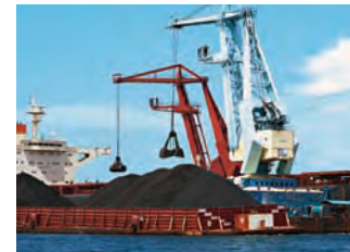
Floating cranes load customer's vessel in the Taboneo anchorage.
