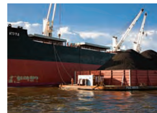
A barge loaded with Envirocoal ties up to a customer vessel that has its own gear.
