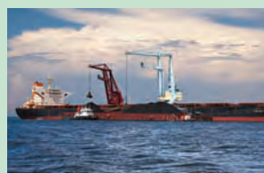
16. Bulk carrier being loaded by floating cranes
