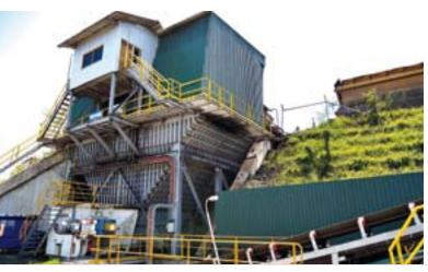
Each single conveyor at Kelanis can load up to 2,000 tonnes per hour on to waiting barges.
